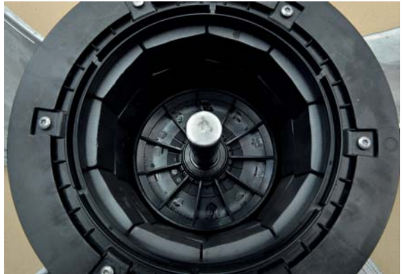
Steel rotor with plastic cooling fan
