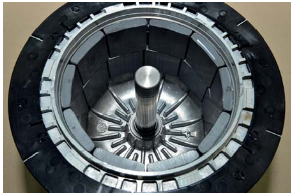
Aluminium die-cast rotor with plastic washer (not shown) on flange
